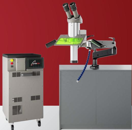
Combo 200 is the Elettrolaser laser system designed to offer maximum flexibility in welding molds and large industrial parts. With its welding head mounted on a long arm extension, it is perfect for working on oversized objects in awkward weld positions, without having to move the workpiece.
