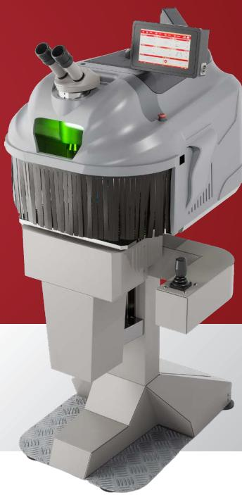
AWL is an automatic laser welder designed for repairing small molds, and precision welding of small medical and industrial components. Equipped with a motorized three-axis (X-Y-Z) table controlled via joystick, it offers precision and accuracy in welding, even in hard-to-reach areas. Available with CNC/ G-CODE programmable option and rotary axis for tubular welds.
